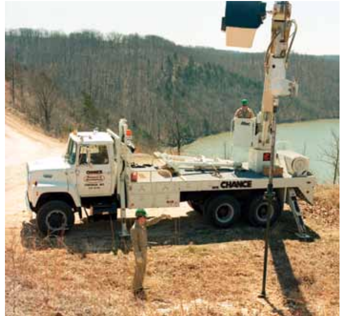
Chance has anchor testing equipment to help utilities plan anchoring requirements.
