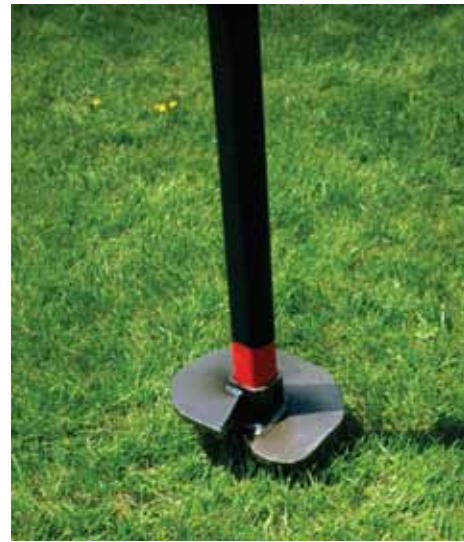
Start anchors in a near vertical position.
