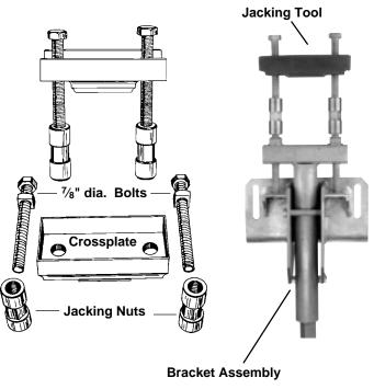
12. Place jack between the T-pipe and the crossplate on the jacking tool. Adjust the height of the jacking tool to match the height of the jack as required.
