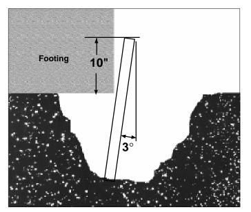
7. The anchor shaft should be terminated with approximately 10 inches of shaft above the footing. A portable band saw may be used to cut the shaft off at the proper height above the footing.
