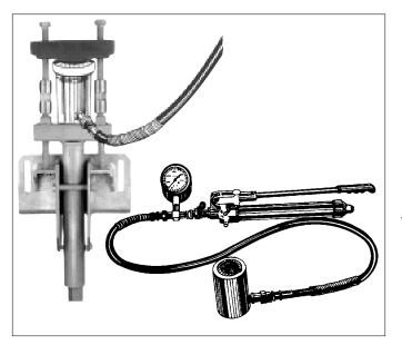
13. Apply a small amount of pressure to jack, just enough to take up the "slack" in the assembly. Once again check to see if the bracket is still mounted flush with the footing. Tighten the crossbolt if necessary and check the anchor mounting bolts again before proceeding.
