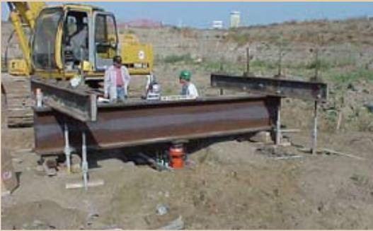
Helical Pulldown® Micropile: Tested to 205 tons
