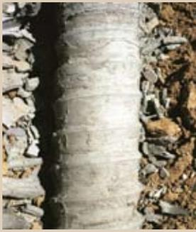
Close-up of Helical Pulldown® Micropile extracted from clay soil
