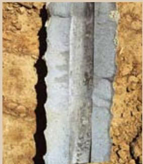
Cross-section of extracted micropile
