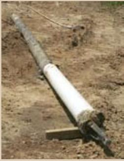
Helical Pulldown® Micropile extracted for visual inspection
